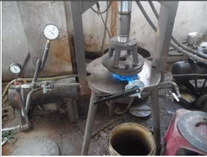
shell strength test
